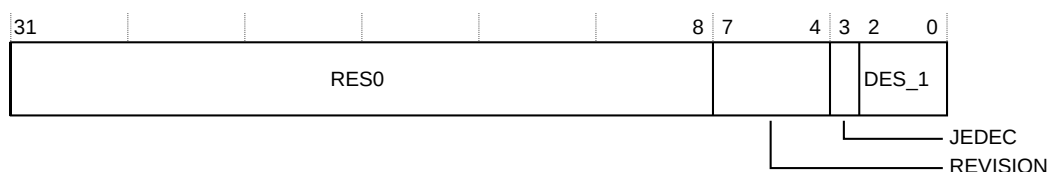
Figure 6-45: PDR2 register bit assignments
